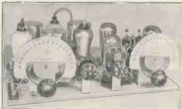
ONLY FOUR KNOBS TO BE MANIPULATED There are only four control knobs on the Welcome Portable—two tuning condensers, volume control, and a combined wave-change and on-off switch
