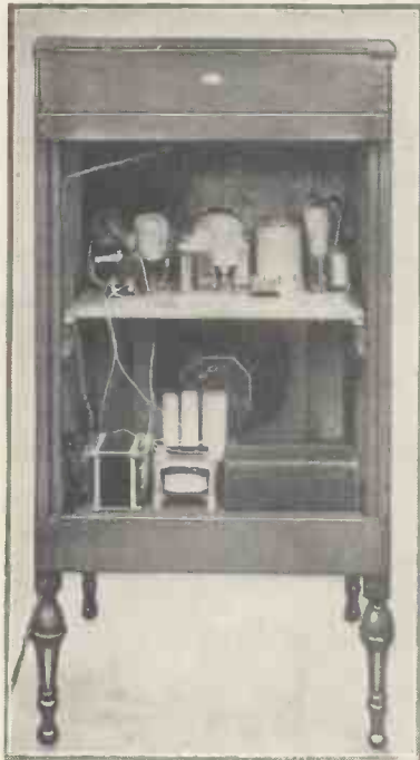
This view of the completed Super-quality Five shows how compact is the assembly. The mains unit is placed on a shelf at the bottom of the Camco cabinet
