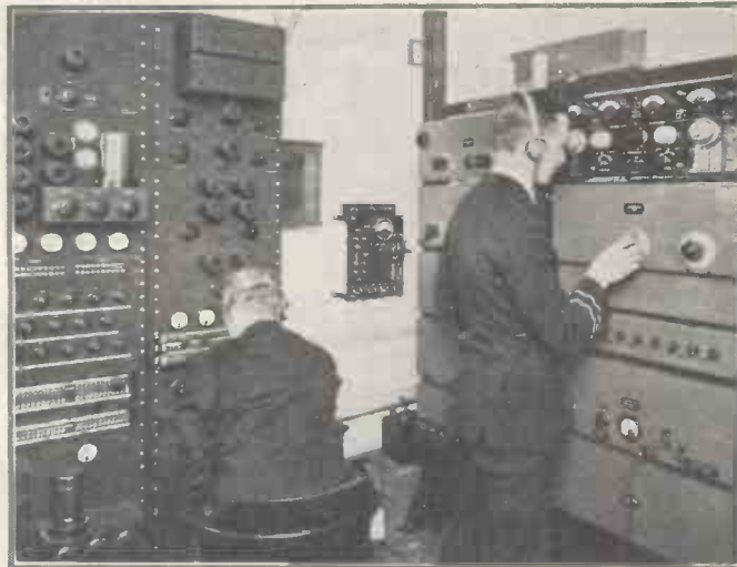
TRANSATLANTIC TELEPHONY ON SHORT WAVES The receiver and terminal equipment installed by the Marconi International Marine Communication Co., Ltd., on the "Empress of Britain"
