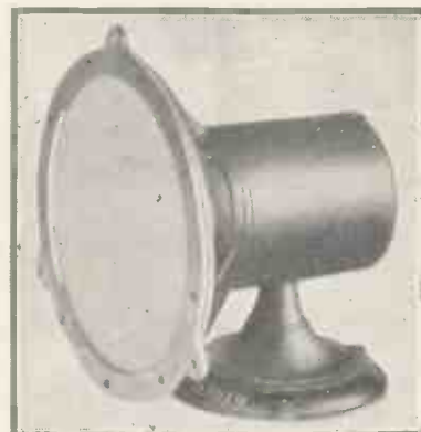
A MOVING-COIL LOUD-SPEAKER One of the first moving-coil loud-speakers. It had a massive pot, enclosed in which was an electromagnetic winding
