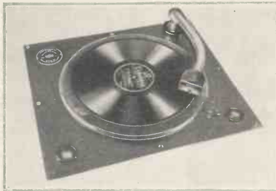
COMPLETE RADIO-GRAMOPHONE FITTING This new Garrard arrangement incorporates an induction motor, a pick-up and volume control, as well as two needle cups, mounted on one plate for fitting in the top of a radio-gramophone cabinet
