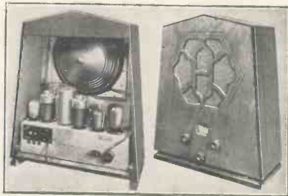
A FINE STRAIGHT RECEIVER A neat walnut cabinet houses the new Six-Sixty Super Five. The large tuning scale is calibrated in wavelengths. A cone loud-speaker is incorporated
