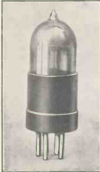
AN EARLY VALVE This valve with a hooded anode was made by Cossor's. It was one of the original dull-emitters
