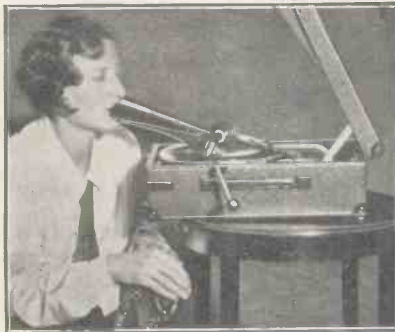
MAKING GRAMOPHONE RECORDS AT HOME A feature of the 1931 Radio Exhibition was a number of home-recording arrangements, one of which is shown in this photograph. This system was purely acoustic
