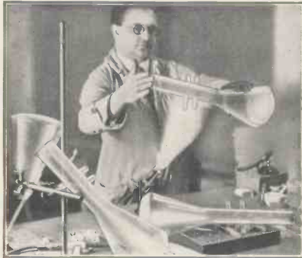
THE MANUFACTURE OF CATHODE-RAY TUBES This photograph of the manufacture of cathode-ray tubes shows clearly the fluorescent screen at one end
