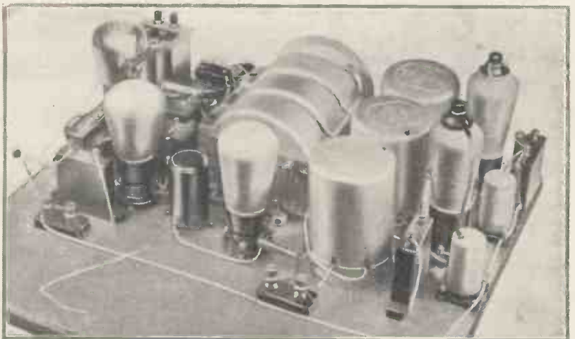
A view of the Super-quality Five with the valves and coil covers in position. Trimming presents no difficulties, and there is only one knob to tune
