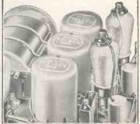
Showing the position occupied by Telsens Triple - Matched Screened Coils in the built-up "Super Quality Five."
