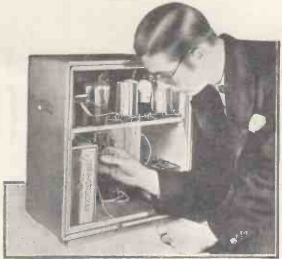
ADJUSTING THE BATTERY VOLTAGES
