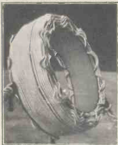
A HOME-WOUND COIL In the early days of broadcasting most constructors made their own coils, of which this is a good example
