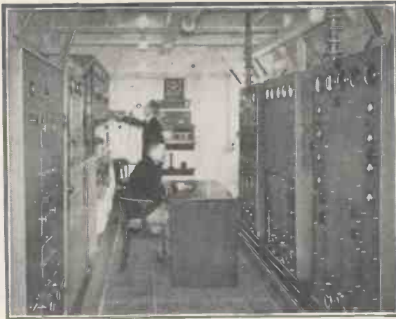
"EMPRESS OF BRITAIN" TELEPHONE TRANSMITTER The Marconi International Marine telephone transmitter, which has a range of 2,000 to 3,000 miles, installed on the "Empress of Britain"
