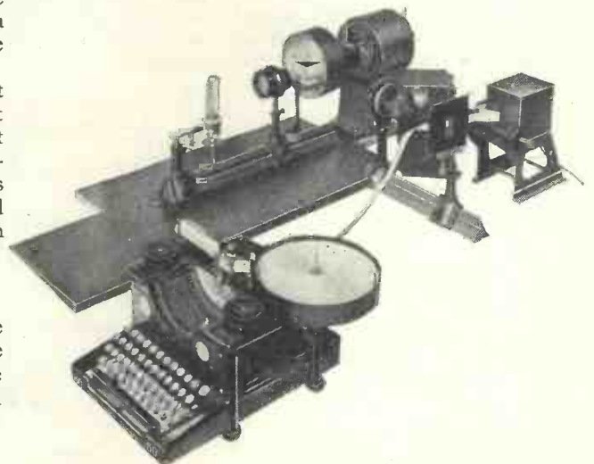
Fig. 5.—Layout of the apparatus for transmitting by television printed characters with the maximum efficiency
