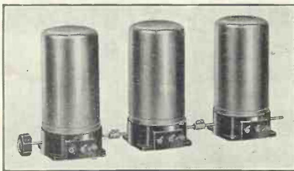
AN ASSEMBLY OF MODERN CANNED COILS This is a group of the latest Tunewell coils. Any number can be combined into one assembly and a single wave-change switch can be used
