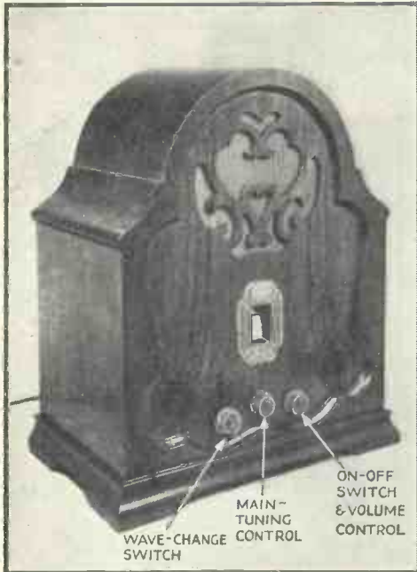
COMPLETELY SELF-CONTAINED This Zetavox receiver needs only an aerial and earth to complete the installation. The appearance of the cabinet is particularly pleasing
