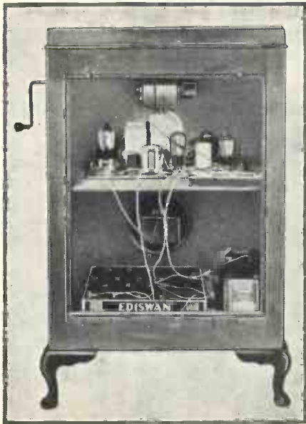
LOUD-SPEAKER AND BATTERIES The back of the Calibrator showing how the loud-speaker and batteries are enclosed in the cabinet
