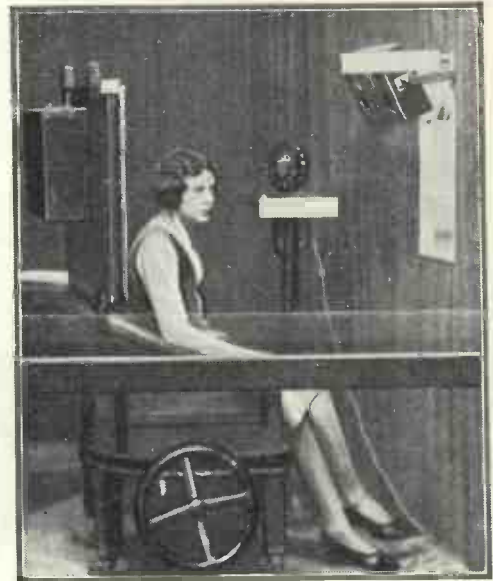
Fig. 1.—The original hand-worked screen news apparatus is seen fixed to the back of the artist's chair in a television studio
