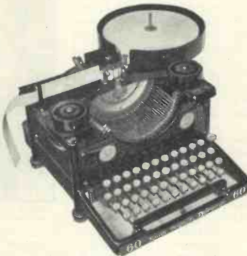
Fig. 4.—Special typewriter built for printing the letters on a paper-tape roll
