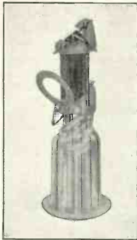
Mica plate bonding employed in the Osram MHL4 A.C. mains valve
