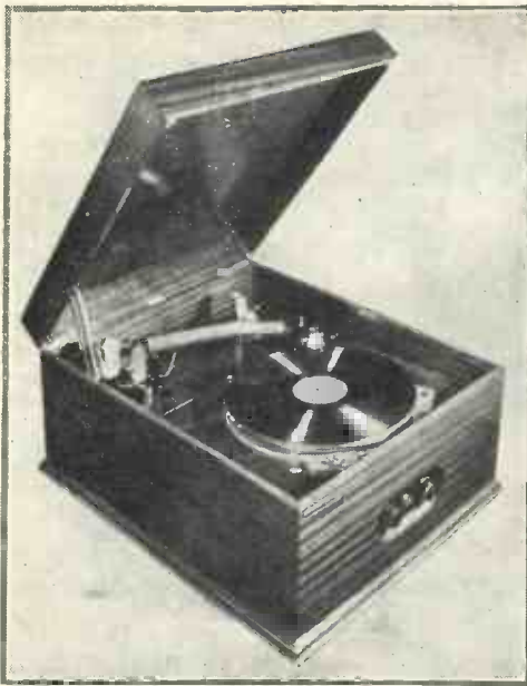
DYNAMICALLY LEVEL PICK-UP Part of the author's radio-gramophone equipment. The pick-up is of a special type and has been set dynamically level
