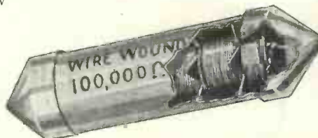
A cartridge type of fixed resistance wound in sections on a bobbin made of an insulating material. The cartridge is held in position in the set by means of spring clips
