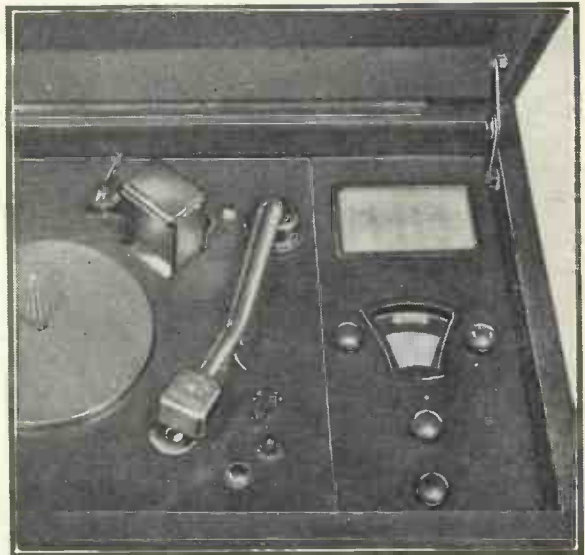
CONTROLS OF A TEN-VALVE SUPER-HET On the right are seen the controls of the H.M.V. Super-het Ten Autoradiogram. The condenser scale is calibrated directly in wavelengths
