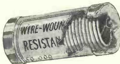
Another type of cartridge resistance, with wire-wound string placed round a cylindrical former
