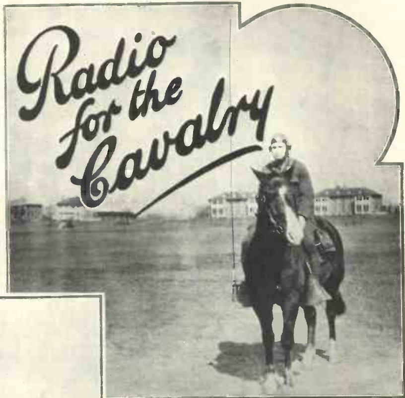
THE HORSE THAT CARRIES A RADIO STATION! An American cavalryman equipped with a radio set that keeps him in touch with headquarters. Note the fishing-rod type of aerial
