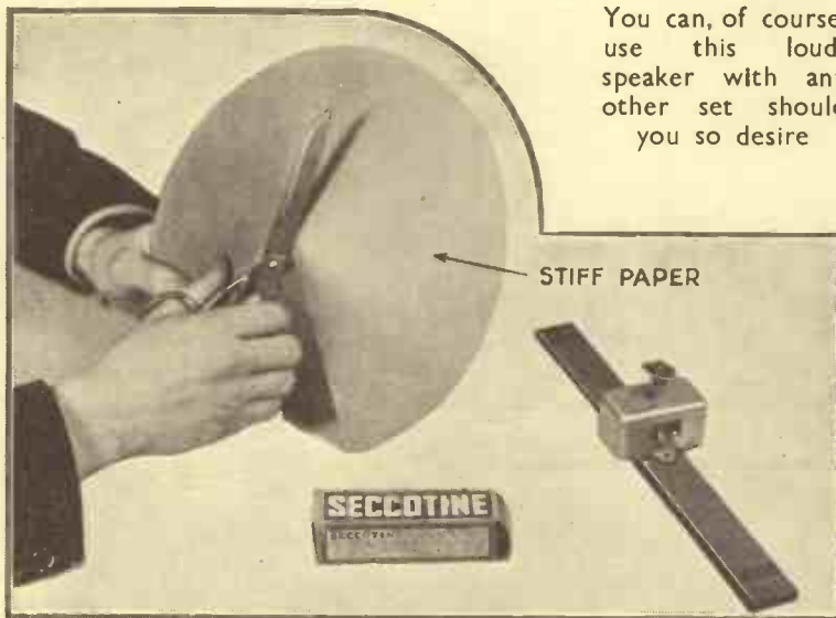
CUTTING OUT THE PAPER CONE DIAPHRAGM
