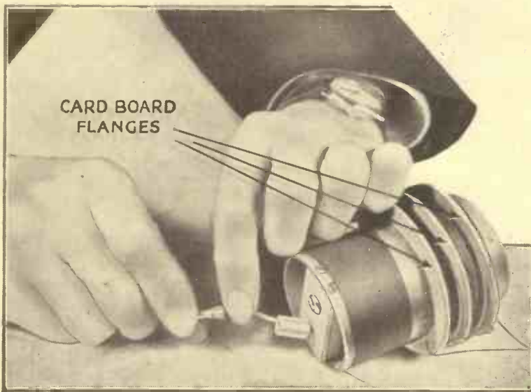
FIXING THE DUAL-RANGE ATTACHMENT
