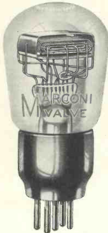
A 2-VOLT BATTERY PENTODE Two-volt battery pentodes are not recommended for general use in C-quality sets, but they can be used in other grades
