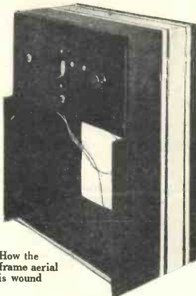
This view shows how the frame-aerial connections are taken to the receiver
