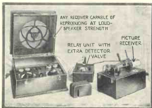
How the Fultograph machine is connected up
