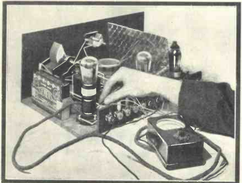
How the Ferranti valve tester is connected in a set. The extra lead is for taking grid-bias voltages
