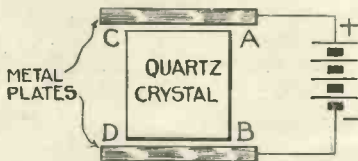
Fig. 1.—Quartz Crystal connected between Two Charged Plates.
