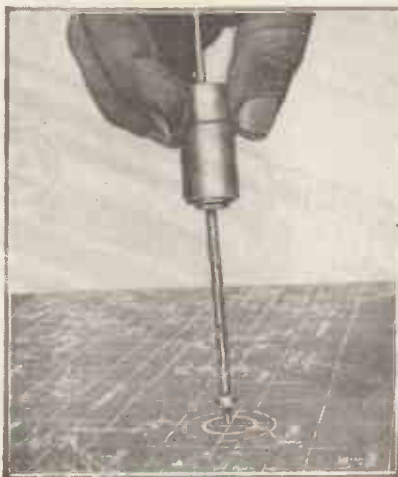
Fig. 22.—Pricking-off with an Auto-centre Punch.
