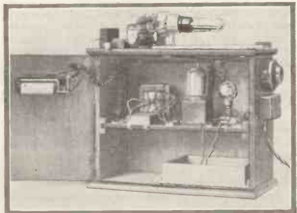
Amplifier for use with the Telegraphone.
