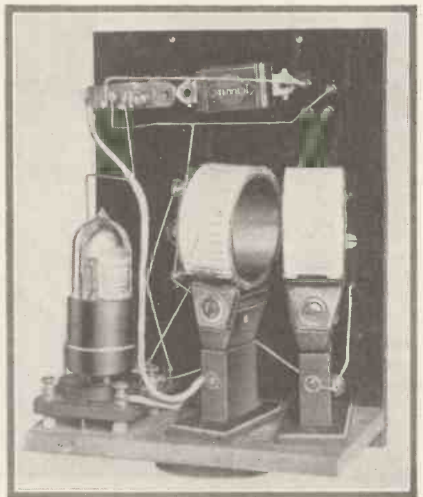
Another View showing Valve and Coils in Position.
