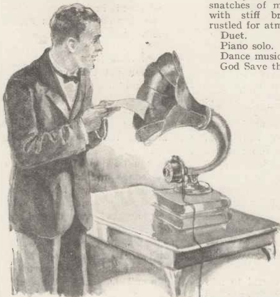
A loud-speaker in the "studio" acts as a microphone for the "home broadcast."
