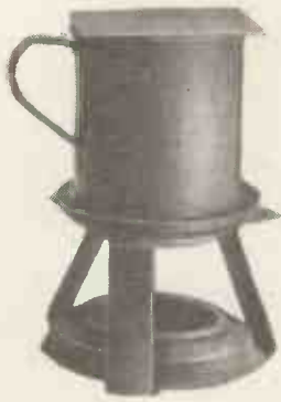
(Above).—A simple outfit for casting sulphur, consisting of an enamelled mug, a sheet of mica, and a spirit lamp.
