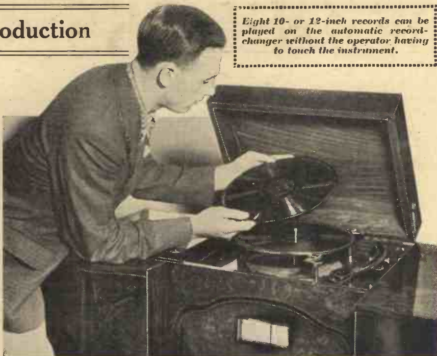
This photograph shows a selection of 12-inch records being placed on the changer.
