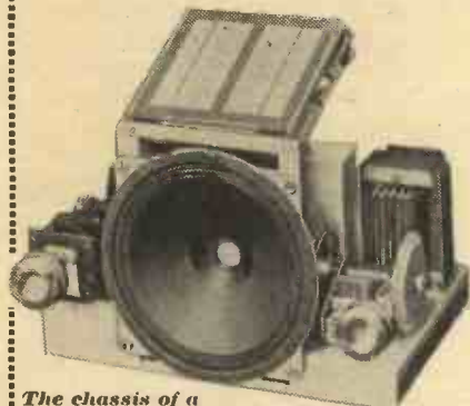
The chassis of a typical low-priced German receiver. It is a two-valve single-tuned-circuit outfit.
