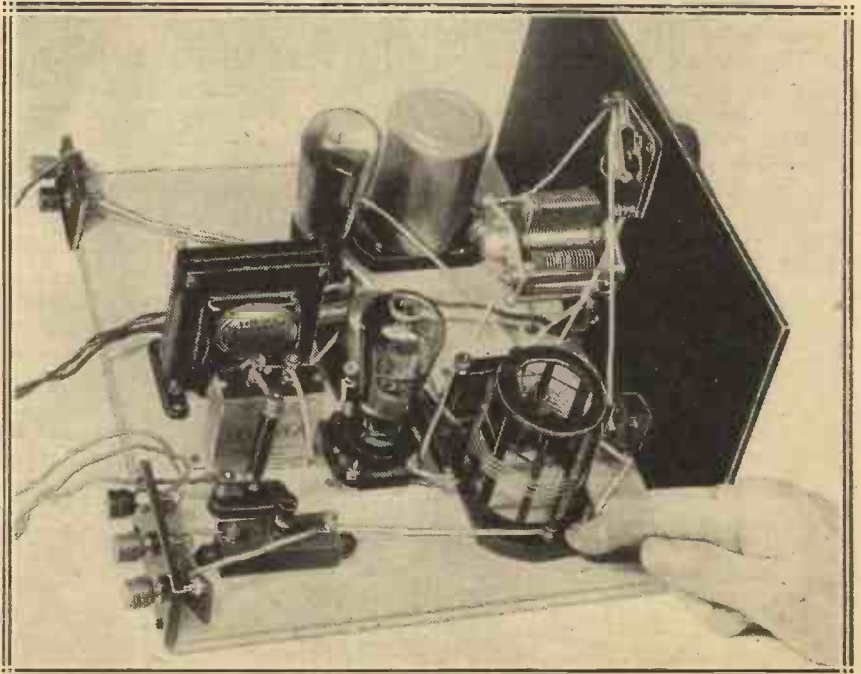
Pointing out the home-wound short-wave coil which is quite independent of the coil for medium and long waves, from which it is well separated. The "broadcast" wave coil is of the screened type, and can be seen on the further side of the tuning condenser.
