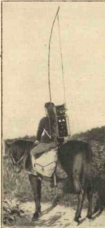
Broadcasting a description of army manoeuvres in Manchuria via a short-wave portable transmitter.
