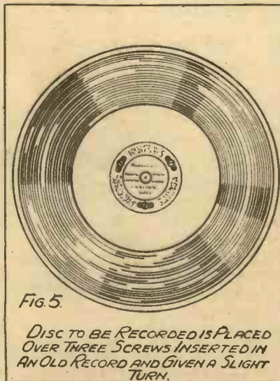
FIG. 5 DISC TO BE RECORDED IS PLACED OVER THREE SCREWS INSERTED IN AN OLD RECORD AND GIVEN A SLIGHT TURN. The disc on which the sounds are to be recorded is securely held to the large record which provides the grooves for the guide needle to run in.
