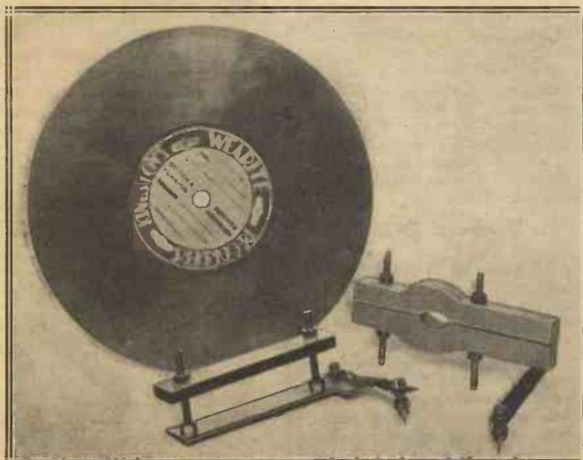
The needles seen in the pick-up clamps run in grooves on a tracking record, and thus move the cutter needle across the blank disc as it is rotated.
