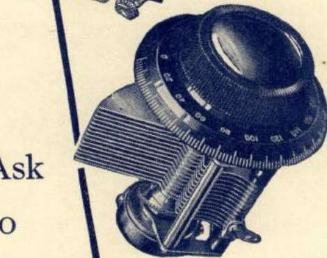
J.L.4 CONDENSER. Specially designed for the S.T.400. Slow-motion type (35/1). Capacity, ·0005. Complete with 3" dial, 7/6. Extra heavy gauge vanes. Rigid nickel-plated frame. High-grade ebonite insulation.
