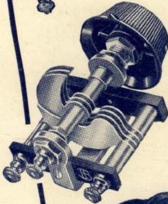
J.L.4 CONDENSER. Specially designed for the S.T.400. Slow-motion type (35/1). Capacity, ·0005. Complete with 3" dial, 7/6. Extra heavy gauge vanes. Rigid nickel-plated frame. High-grade ebonite insulation.
