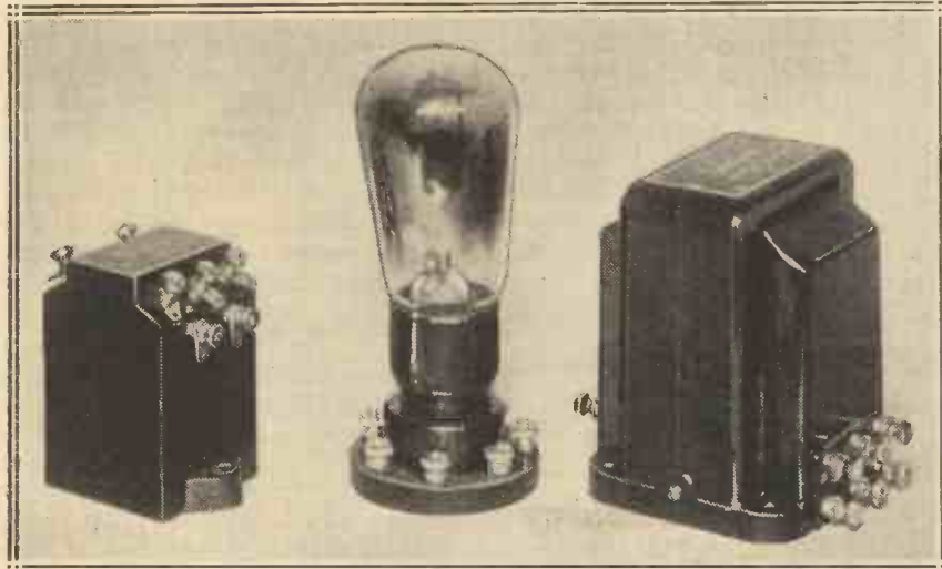
THE "RAW MATERIAL." —The three main components needed for practical "Class B" working are shown separately here. On the left is the Varley driver transformer with alternative ratios of 1:1 and 1.5:1; a "Class B" valve in its holder is in the centre; with a special output choke on the right.
