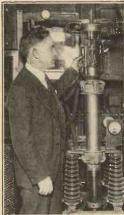
America's biggest transmitting "tube"—a 200 kilowatt—is here being contrasted with one of the ordinary receiving type.
