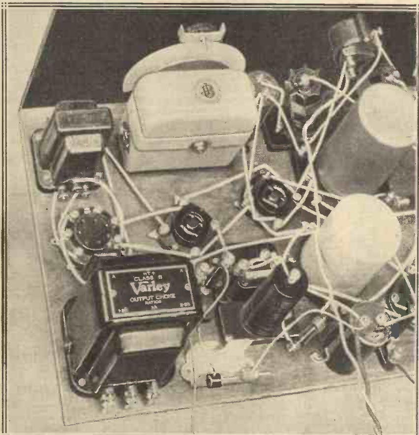
Between the panel and the 7-pin "Class B" valve holder is the special drive transformer operated by a small power valve which goes into the adjacent valve holder.
