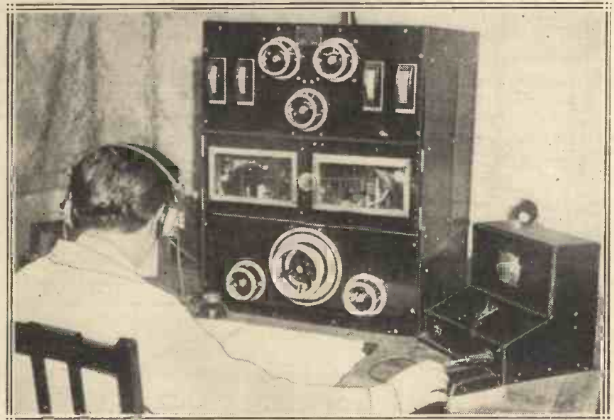
Police authorities everywhere are developing fresh uses for radio in curbing the activities of criminals. A recent innovation is the installation by the Paris police of a special transmitter capable of sending by wireless photographs of wrong-doers, together with impressions of their finger-prints.
