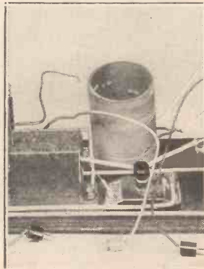
Coils should not be mounted like this when a metal-covered baseboard is used, as the presence of the conductive surface reduces the effective inductance of the winding. In such cases it is better to fix the coil in a horizontal position, well away from the baseboard.
