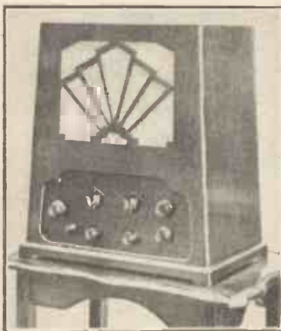
Here is a front view of the all-from-the-mains version of the "S.T.300," as described in the accompanying letter from Mr. Cavanagh. He drives the loudspeaker (shown in the opposite photograph) from a pentode.
