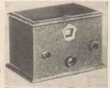
By the addition of this simple unit you can transform an old unselective receiver into one comparable with a really up-to-date model.
