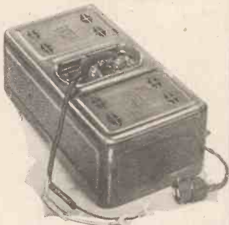
The Ekco K.25 A.C. mains unit is designed to give a high-tension output of 25 m.a., and is also provided with a switch for trickle-charging the L.T. battery.
