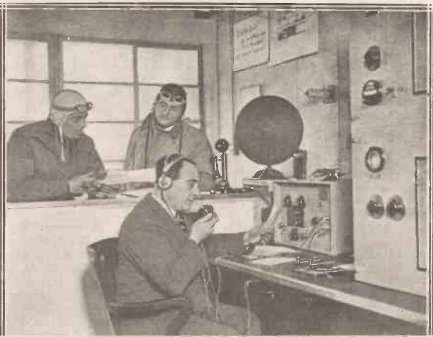
The Automobile Association (more generally known as the A.A.) has developed a weather report service for private owners of aircraft. The photograph shows the radio transmitter used for the broadcasting of the reports which are sent out at regular intervals on a wave-length slightly above 800 metres. This station is the first of a series to be erected throughout the country.
