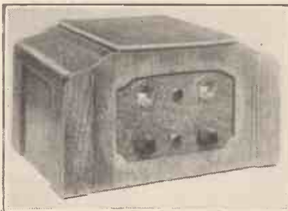
The "Meteor" 3 is an efficient three-valver designed to work on three wave-bands; viz., short, medium and long. The tuning and reaction condensers are both fitted with slow-motion drives.
