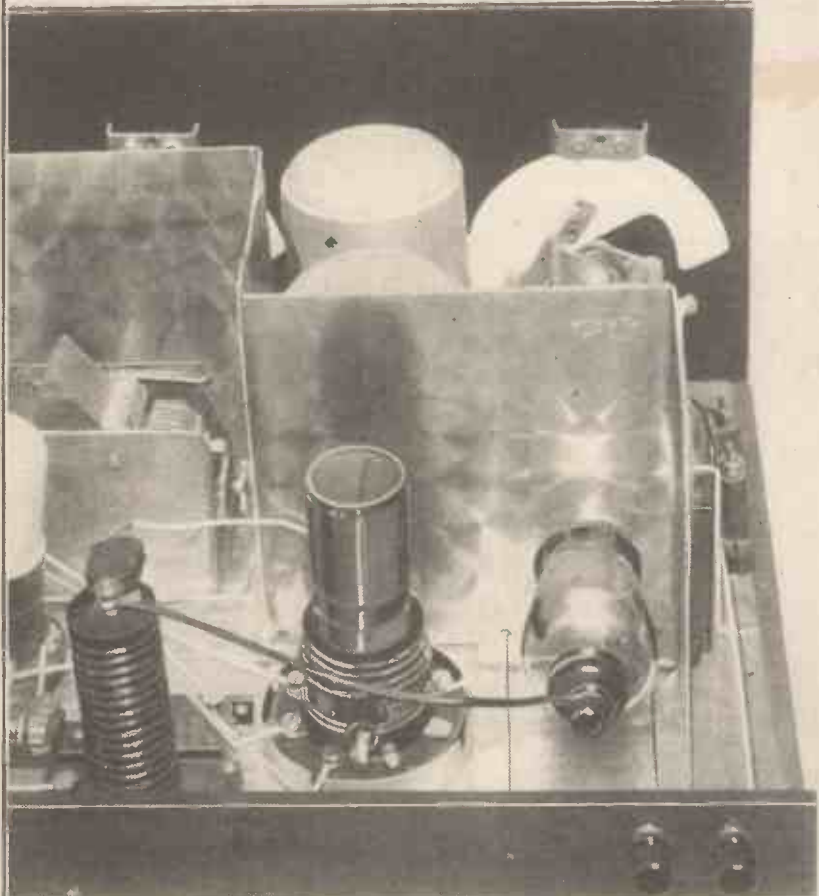
The special shaped vertical screen prevents all howls and other forms of H.F. instability. The metal cover has been removed from the coil in the foreground.
