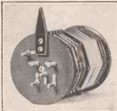
The little piece of pointed ebonite is the only addition needed on the coil, but by means of it a condenser is shorted as the coil is inserted into its holder.
