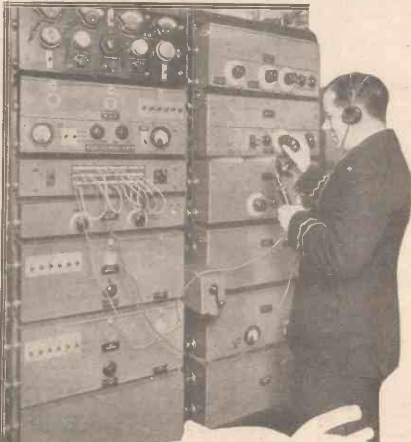
The "Homer" keeps in touch with land by means of short waves. Here is the short-wave receiver.
