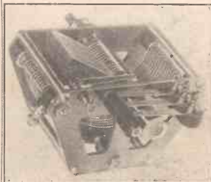
This view of the "Cyldon" Extenser shows the arrangement of the self-changer contacts. Note that the rotation of the cam renders the phosphor-bronze collector brushes self-cleaning.
