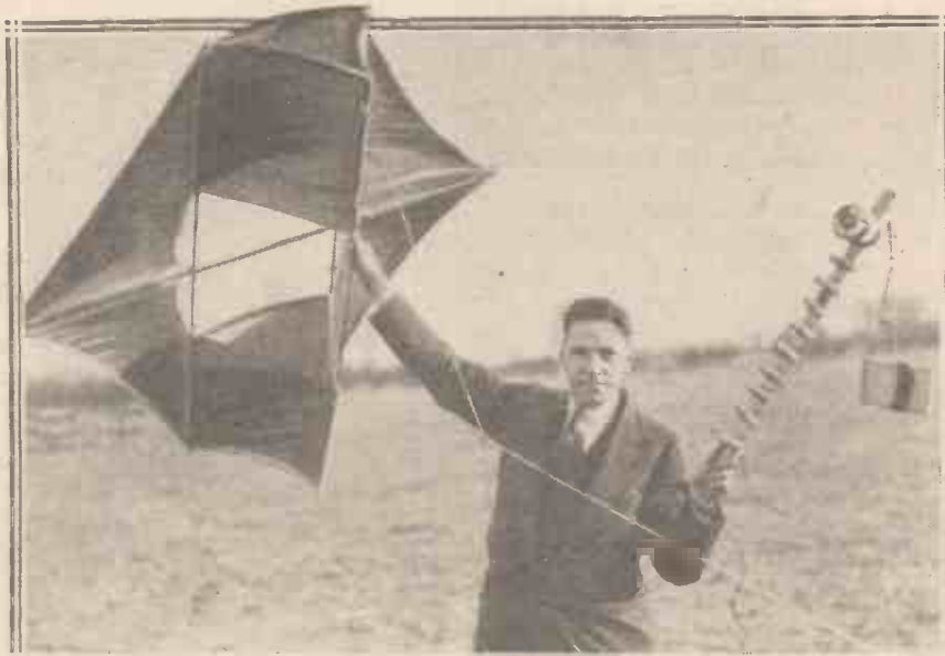
An engineer at the Radio Research Station, Slough, with one of the kites used for special radio tests. They take up about 100 ft. of aerial wire and very small transmitters.
