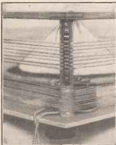
Here you see the long-wave frame above the medium-wave frame, and you will see quite clearly how the former is wound in slots on special corner-pieces.
