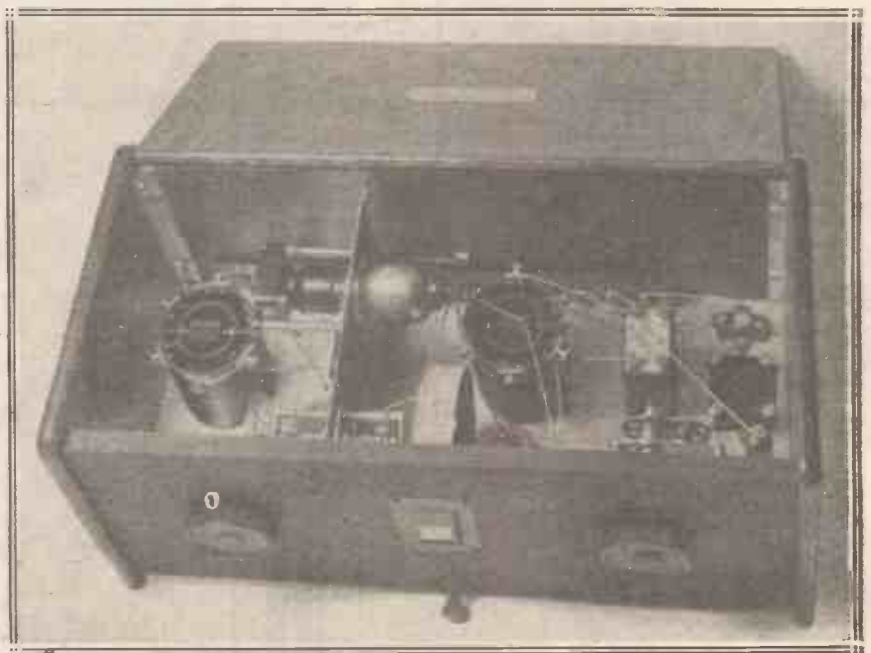
A view showing the inside and general arrangement of the Osram "Music Magnet," as made up from the kit of parts.
