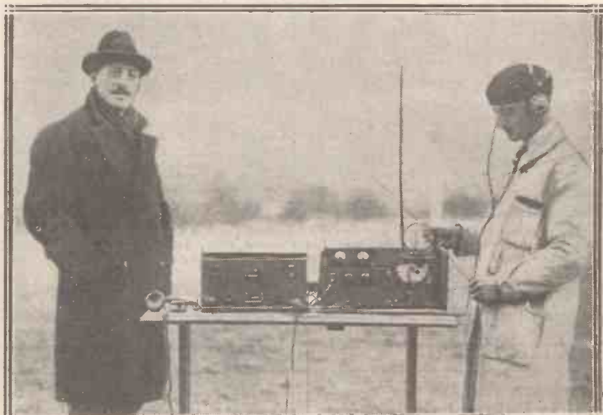
To the right of this photograph is M. Beauvais adjusting an instrument which he has invented for overcoming parasitic noises, such as atmospherics. M. Beauvais is already well known as the originator of a scheme for guiding aeroplanes by wireless.
