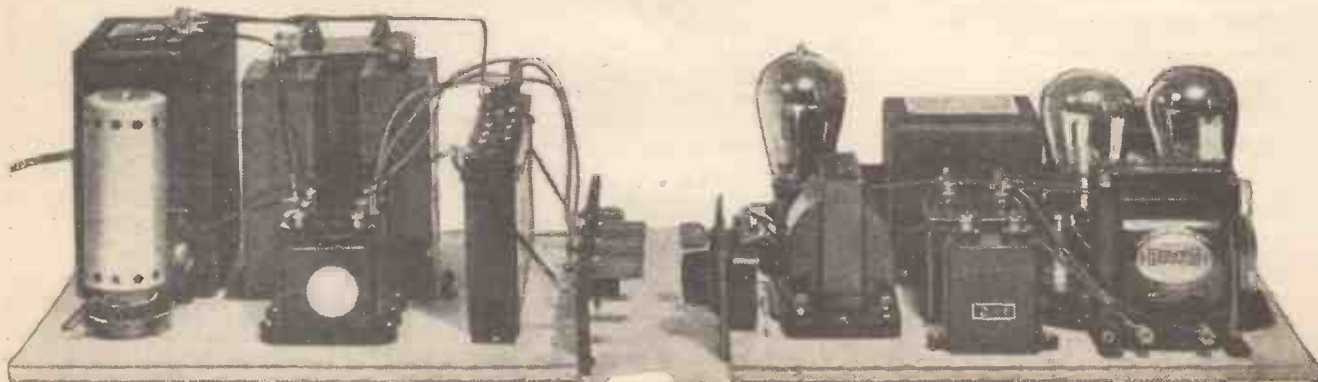
The H.T. power unit and the amplifier section of the All-Electric Gramophone.
