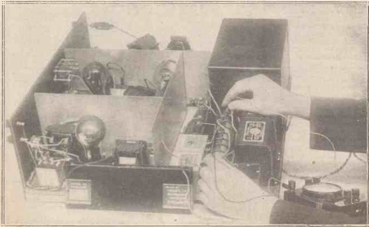
Measuring the voltage across the various H.T. tappings with a high-resistance voltmeter.
