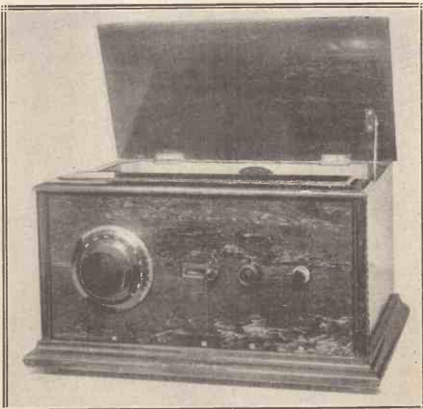
Apart from the wave-change switch, the controls are similar to those used on any ordinary straight two-valve set.
