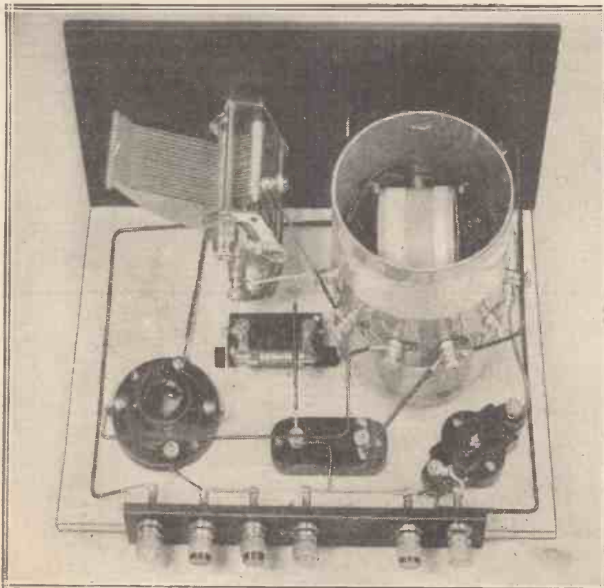
A vario-coupler type of reaction control is employed, while a wave-change switch is also incorporated in the tuning unit.
