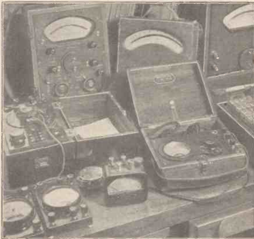
Some of the apparatus used in the "Wireless Constructor" laboratory. The milliammeters in the left foreground are useful for taking valve curves and testing for overloading, while the meter on the right is a complete set tester that is often found extremely valuable.
