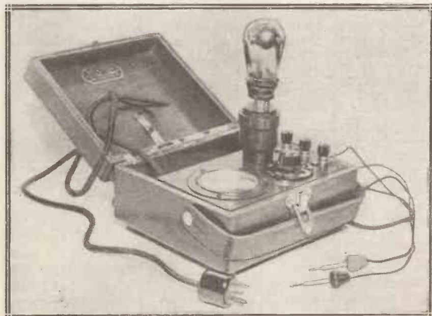
A Weston set tester which is invaluable for tracing faults. Every circuit can be tested in a very short time.
