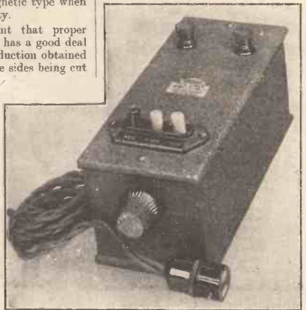
One of the "Elco" H.T. units (for use on D.C. mains) described in the January issue of the "Wireless Constructor."
