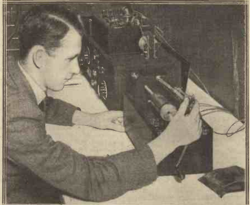
Transmitting the first Fultograph picture from Savoy Hill, whence it was "landlined" to 5 X X and there sent by radio.
