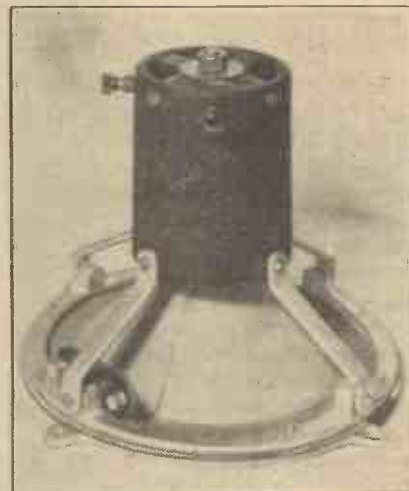
Another view of the "Sylphone" speaker showing the ventilation provided at the back of the instrument for cooling the "pot."
