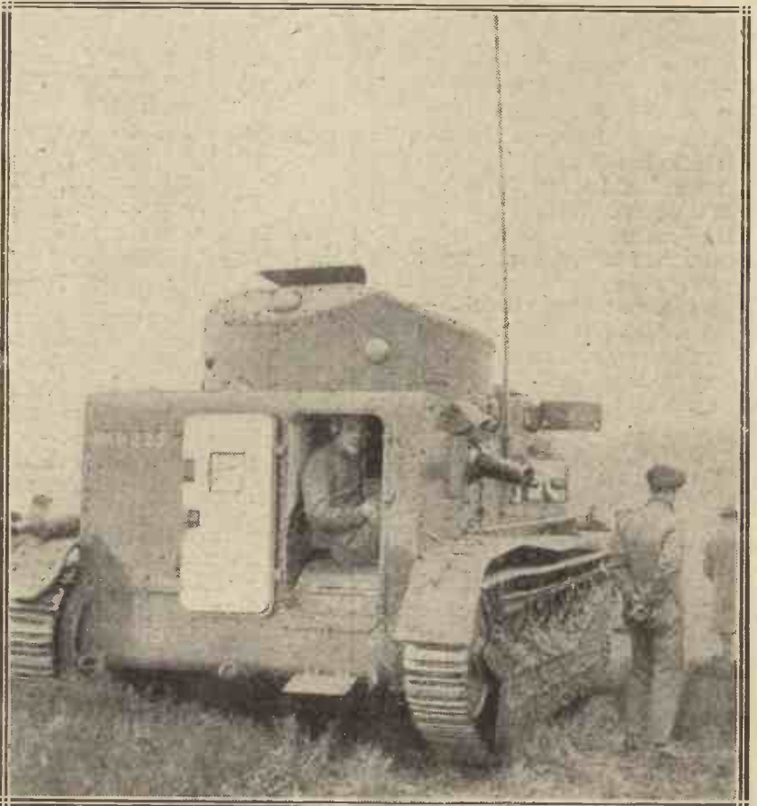
It requires a good operator to read Morse correctly in these conditions. One of the latest "Whippet" tanks, showing the radio-man's quarters.
