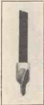
The combined drill and countersink that is described in this column. It is easily made and is an extremely useful gadget.
