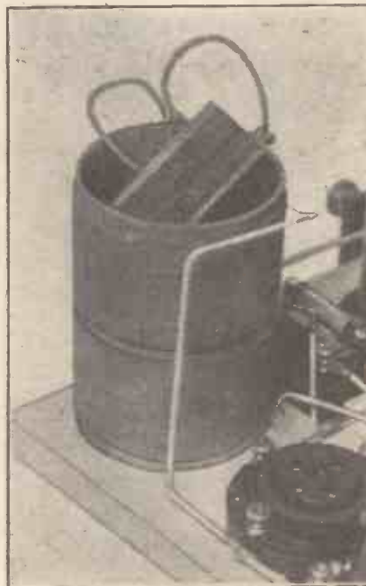
The special astatic oscillator coupler designed specifically for this set.
