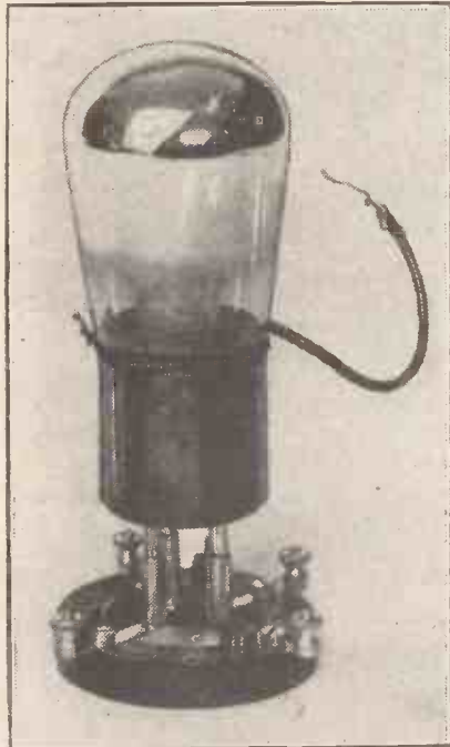
Instead of the flexible lead shown here, the new Interdyne valve sold by R.L. Varley, Ltd., has a small terminal on the base of the valve.
