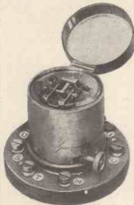
A Post Office "A" type relay.
