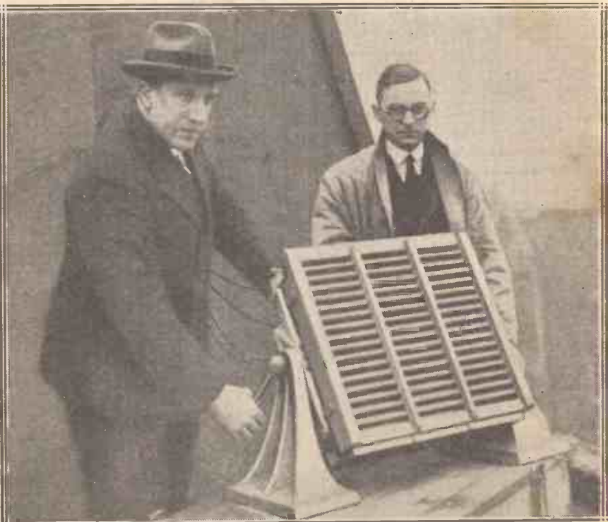
This super-loud-speaker, which was recently brought over from the Continent, operates on the "moving-coil" principle. It is driven by a 1,500-volt generator and makes a greater noise than the Albert Hall organ. In the open country it can be heard over a distance of five miles.
