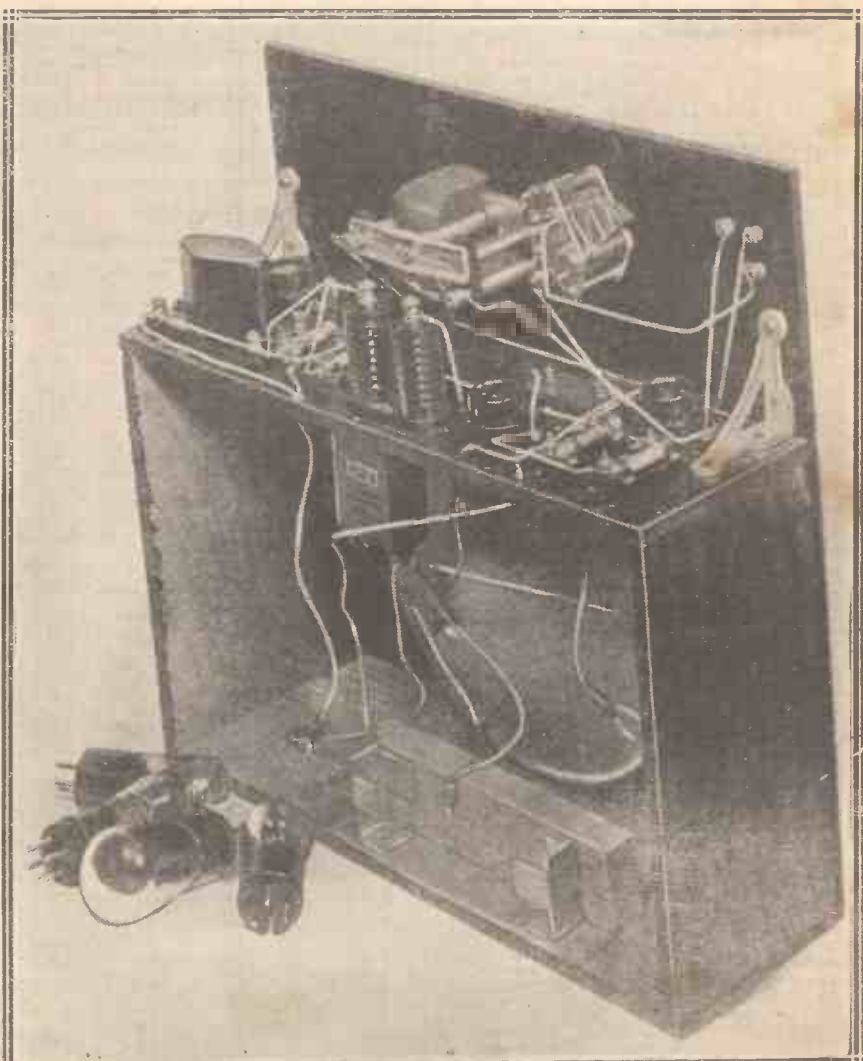
The design of the set is so arranged that the batteries can be removed for inspection or renewal in a few moments, without having to fiddle about among a lot of wires and odd components.
