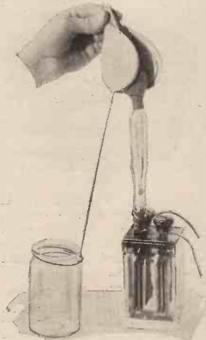
The hydrometer can be left in position during the process of charging. To take a reading all that is necessary is to compress the clip, which releases the bulb and allows the glass tube to fill.
