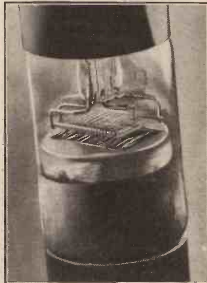
The peculiar internal construction of the Cossor screened-grid valve is shown above. Note the rectangular slot in the screen with its mesh "grid." So far we have been unable to give this valve a thorough test.
