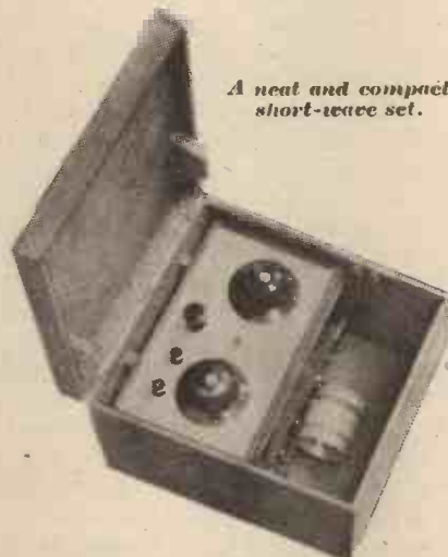
The R.I. Varley short-wave portable receiver, which operates from a collapsible vertical aerial.
