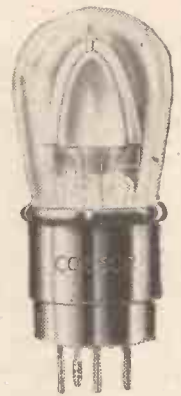
A famous 2-volt power valve—the "Stentor Two."
