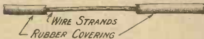
Fig. 2.—When baring flex wires, leave a piece of insulation at the end to keep the strands together.
