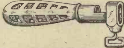
Fig. 5.—This type of universal file handle forms a convenient grip for files or other small tools.
