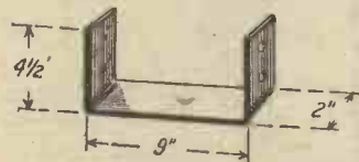
Fig. 2.—Details of the strip of iron which acts as a stop when the mast is erected.
