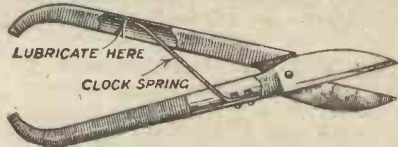
Fig. 2.— By fitting a spring to the handles, shears can be made to open automatically.
