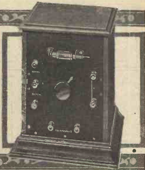
A selective crystal receiver employing a variometer in a novel manner.
