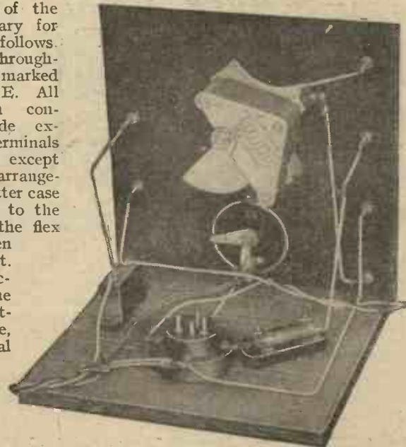
Another back of panel view. Note the flexible leads on the left which go to the batteries.
