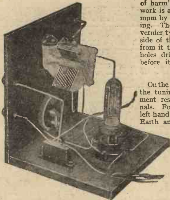
An interior view of the receiver. The phone condenser is in the foreground.
