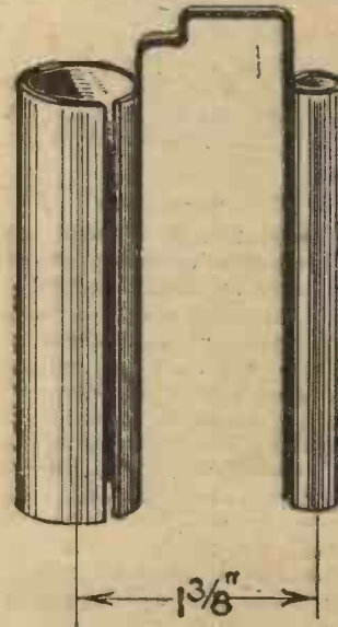
Fig. 2.—A pair of plates after bending to shape.
