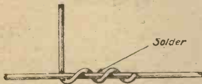
Fig. 1.—A simple joint with round wire.
