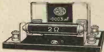
Grid Condenser and Leak mounted
