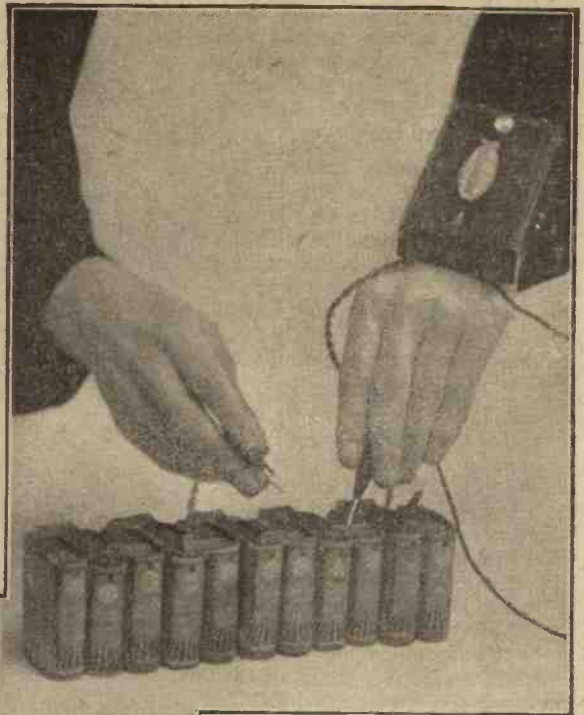
Testing H.T. battery units.
