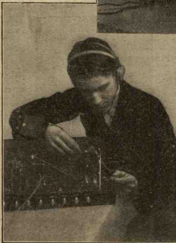
Finding a fault in a variable condenser.
