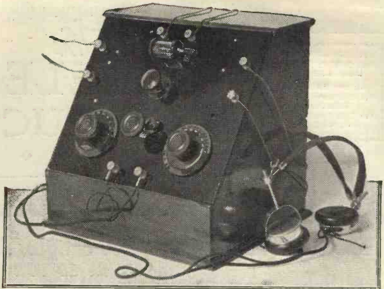
Ready for work. The knob immediately below the crystal detector controls the filament resistance. Reaction is varied by the lower knob.
