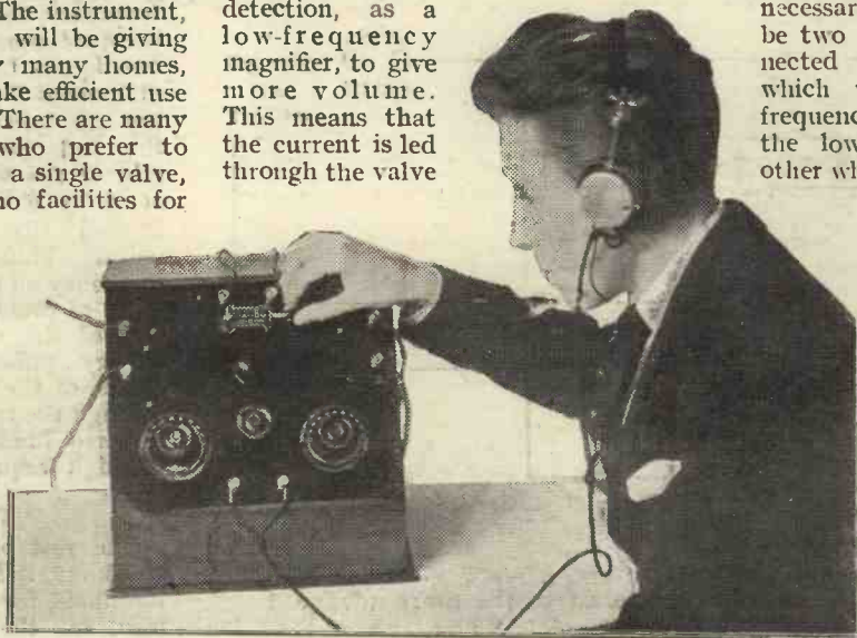
The valve and tuning coils are concealed within the cabinet. All adjustments are made from the outside.
