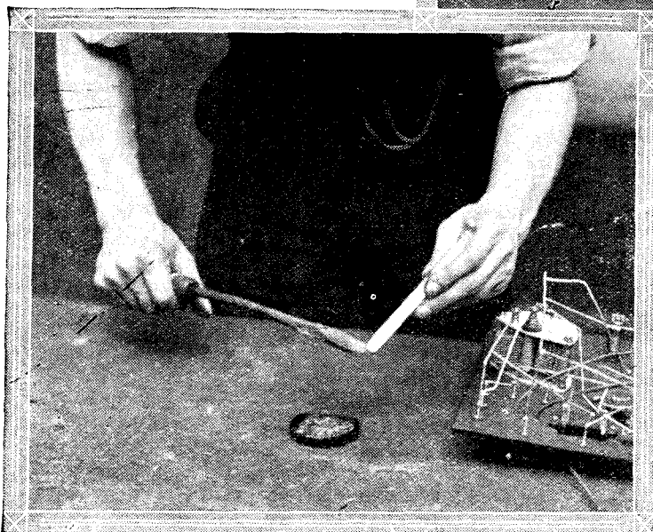
Fig. 3.—Applying the solder.
