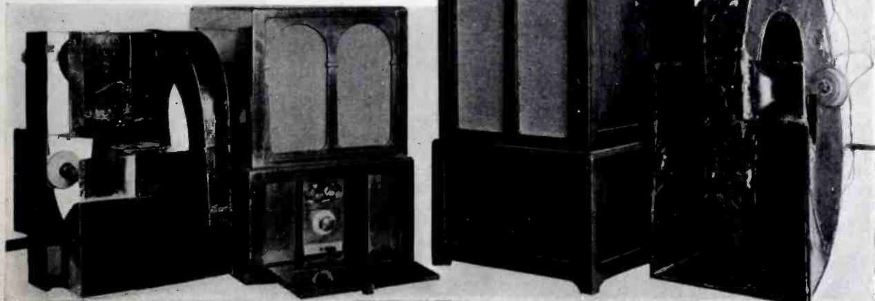
Figure 5—The Triplette horn bent and fitted into a cabinet
