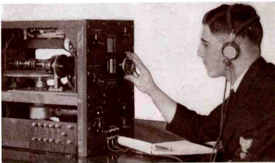
The sonic depth-finder installed aboard the "Tampa" to locate icebergs—it employs sound waves and radio waves in its operation
