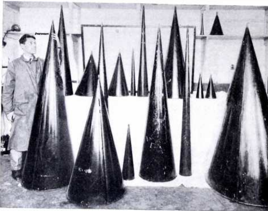
Various sizes and designs of the conical type of horn experimented with
