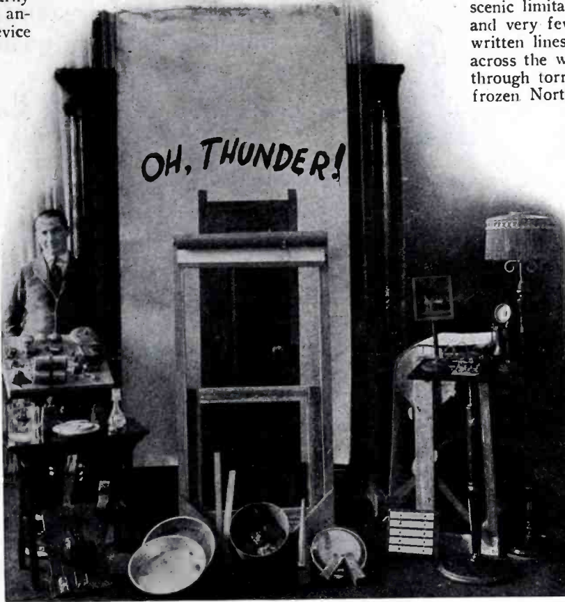
The devices used in a radio broadcasting station in broadcasting drama. Note the portable door and bell-board for delivering sound properties
