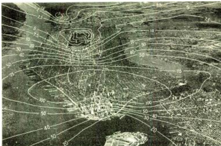
The field of radio waves as affected by conditions in New York City
