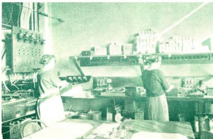
Figure 3—Testing for electron emission, state of vacuum and general operation of tube
