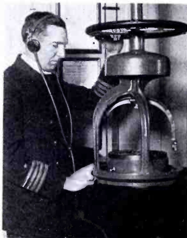
Staff Commander, H. C. Fish, of the S.S. "Leviathan," at the radio compass through which the location of the ship may be ascertained even when the fog is so dense that the sun cannot be seen.
