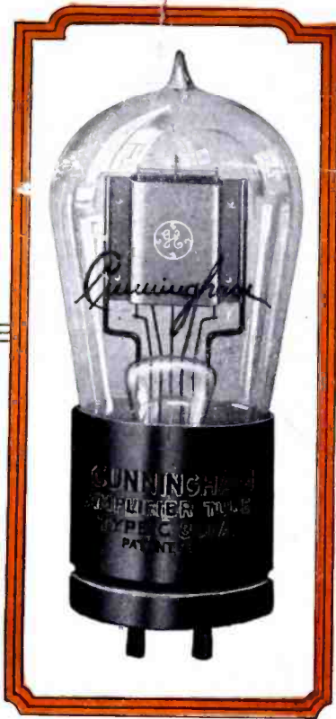
Type C-301A gives greater Power Amplifica- tion with only \frac{1}{4} Amp. Filament Current.
