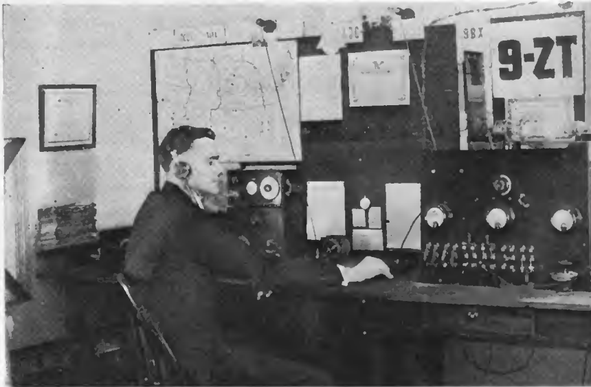
Tube transmitter and receiving equipment of amateur station 9ZT, owned and operated by D. C. Wallace, Minneapolis, Minn.
