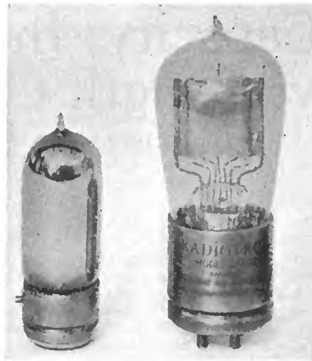
Figure 9—Comparative size of Radiotrons UV-199 and UV-201-A
