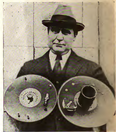
Crystal receiving sets mounted on old phonograph record discs by W. J. Simpson
