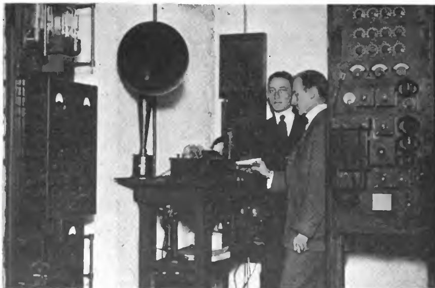
When the President addressed the special session of Congress that convened on Nov. 20, this apparatus in the basement of the Capitol was used to amplify the currents from the microphone in the House of Representatives. From this Western Electric installation, directly under the historic chamber, wires led to the Navy radio station, NAH, for broadcasting the President's voice so all could listen
