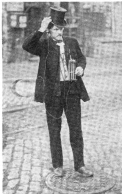
With a receiving set carried in his hat and using a guy wire for antenna and man-hole plate for ground, Frank Chambers listens in on radio traffic
