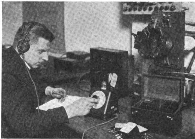
Miniature wireless 'phone and telegraph outfit which is now used on board ships in Germany
