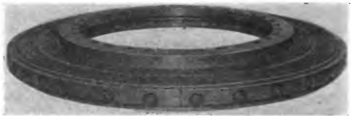
Figure 9—Completed armature ready for sawing into two sections
