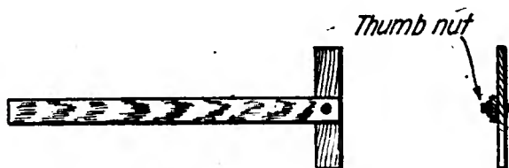
Figure 4—Method of constructing the alidade
