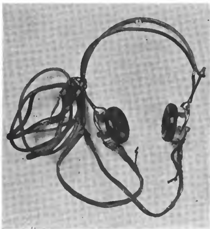
Figure 10—Shielded telephone head set with flexible Belden braid wire cord
