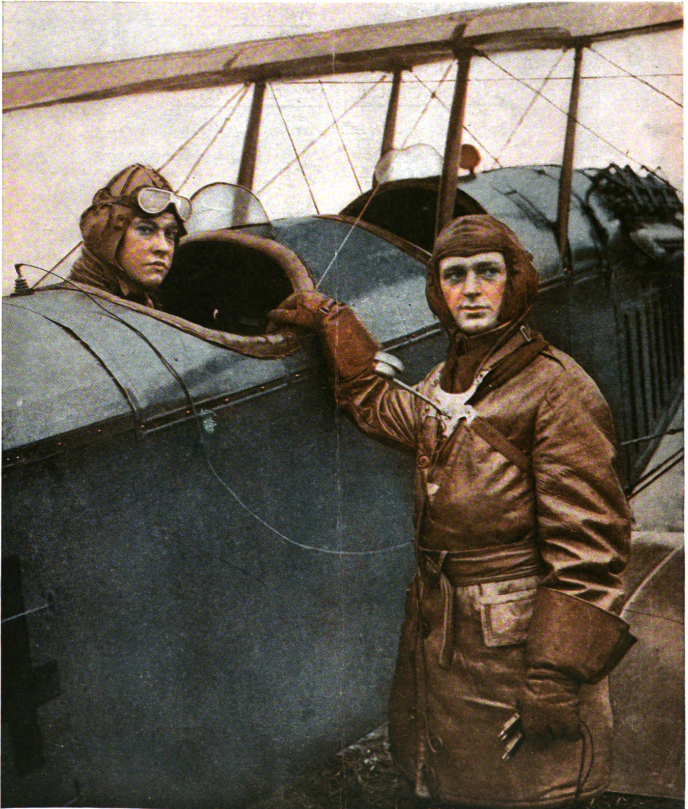
An Aviator's Wireless Telephone Equipment Showing the Transmitter and the Receiving Helmet
