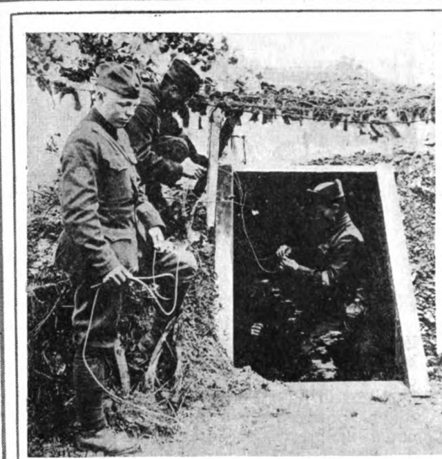
To the right: A signal Corps official photograph of the light microphone set used in trench eavesdropping operations which have been so widely discussed by home-coming soldiers. The apparatus can be used for either local underground or surface listening and the observer may be placed any desired distance from the point of detection
