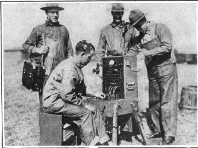
The Marines, too, have their signal units; here they are shown grouped above a telephone switchboard used at division headquarters
