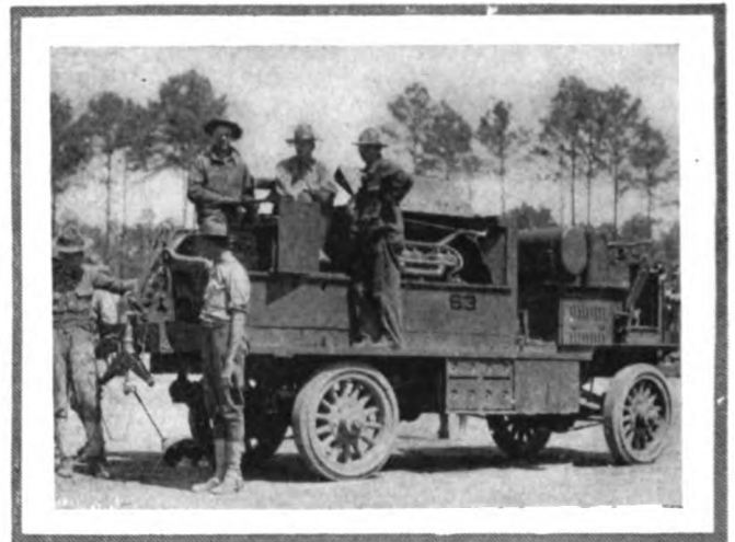
When the observation balloon is to be lowered the engine installed on the bed of this truck operates a winch around which the steel anchor cable is wound
