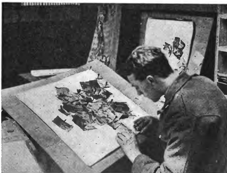
This view shows how the snapshots are assembled to make an accurate map of the enemy territory for staff use. The assembler uses as a guide a military outline map
