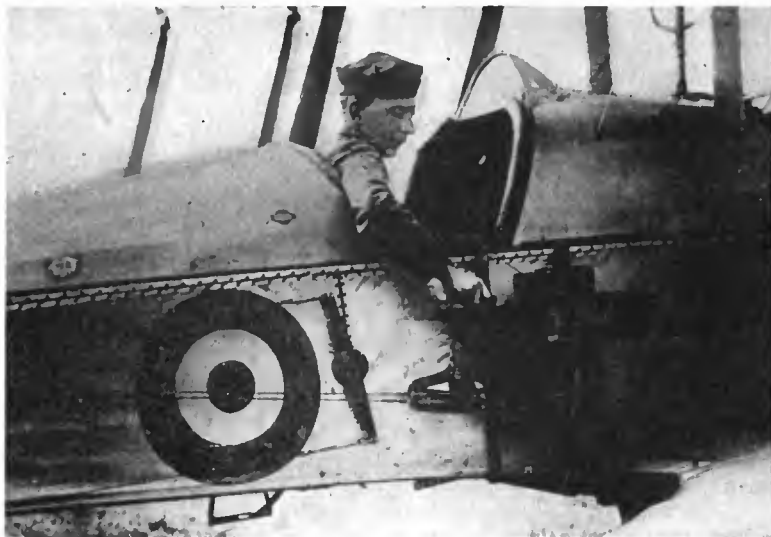
The method of taking observation photographs is shown in this view of the aviator snapping the shutter of the camera fastened to the side of a tractor airplane
