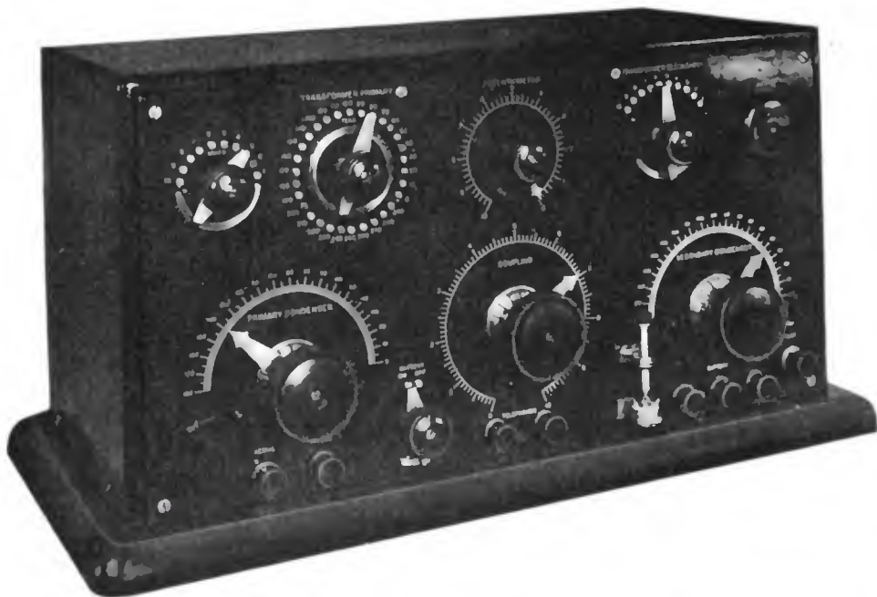
Figure 134—Front view of the Marconi type 106 receiving tuner. The two switches on the front marked "Transformer Primary" vary the inductance of the primary circuit. The switch marked "units" cuts in a single turn of the primary coil at a time. The switch marked "tens" varies the primary inductance in groups of ten turns at each point of contact. The primary condenser is connected in series with the antenna circuit. The switch marked "transformer secondary" and the control handle marked "secondary condenser" control the inductance and capacity of the secondary circuit. The control handle marked "potentiometer" varies the flow of current through the detector. The switch marked "battery" turns the local battery current on and off. These terminals are connected to four dry cells in a separate box. The terminals marked "telephones" are the binding posts for connections to 2,000 ohm telephone receivers.
